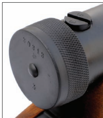
The end cap holds the guide rod and the red polyurethane buffer pad. The receiver is held to the butt and trigger housing by the large threaded takedown bolt.
