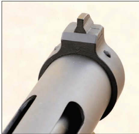
The front sight blade can be drifted in its dovetail for windage adjustment on a steel band wrapped around the front end of the barrel jacket and retained by a crosspin.
