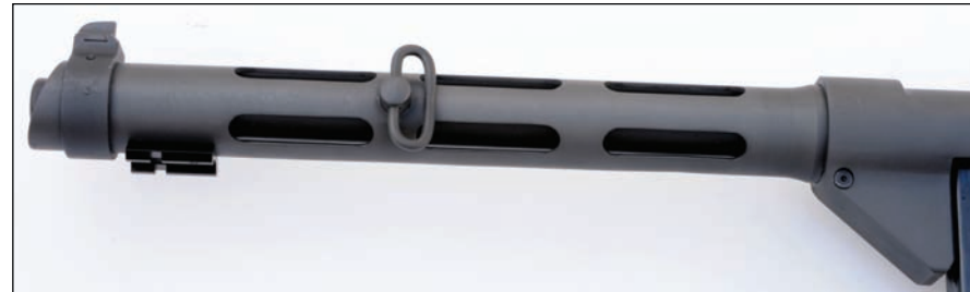
The barrel is held in place by the barrel jacket. These were of dubious value for cooling, but did protect the hand from a hot barrel and the barrel from damage.
