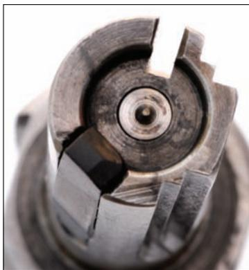
**The Finnish m/31 Suomi's bolt breechface features a firing pin that can be replaced, if necessary, as it was press-fit in place and not milled into the breechface.**
