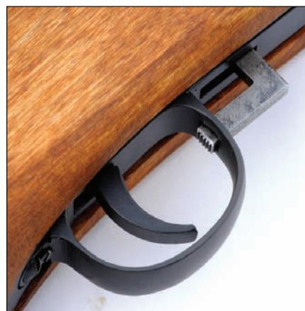
**Push the selector bar fully forward for full-auto fire. Fully rearward, it blocks the trigger. Moving it to the middle position will yield semiautomatic fire.**
