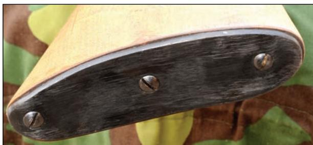
**The steel buttplate has no serrations and the weapon is quite heavy, so the Suomi will sometimes slip out of the operator's shoulder pocket during burst fire.**
