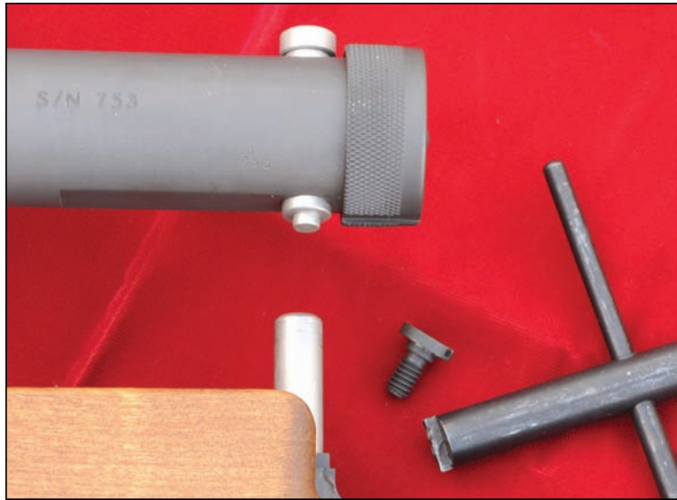
A stainless steel rear post is now attached to the stock group. It has been threaded and counterbored to accept the new and much shorter takedown keeper screw.
