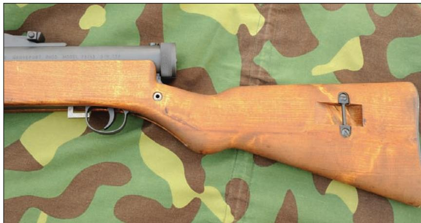
**The Finnish m/31 buttstock is made of beech. This appeared unissued. These sometimes cracked at the wrist area because of the SMG's substantial recoil impulse.**
