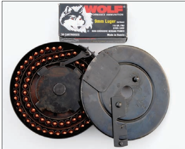
Finnish m/31 Suomi and Russian PPSH41 drums are almost identical in design and can be loaded to full 71-round capacity or with any lesser quantity of ammunition.
