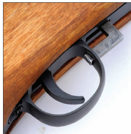
Push the selector bar fully forward for full-auto fire. Fully rearward, it blocks the trigger. Moving it to the middle position will yield semiautomatic fire.
