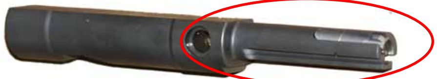
Bolt Face, Extractor Pocket, & Bolt Body
