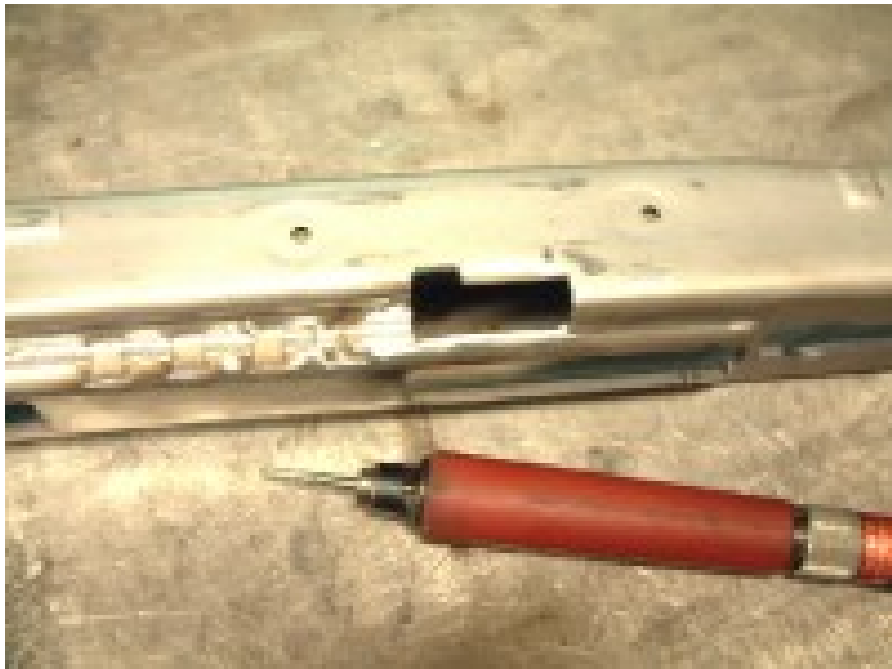
16: Clean up the cut out and slot. Trial fit charging handle.
