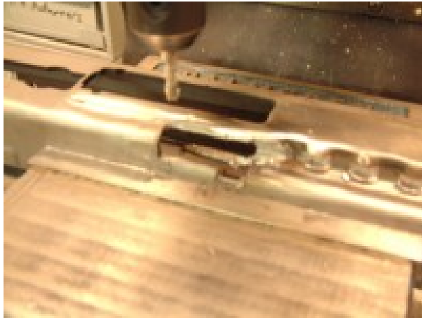
15: Mill charging handle cut out. You will need to rotate the receiver to complete the cut out.
