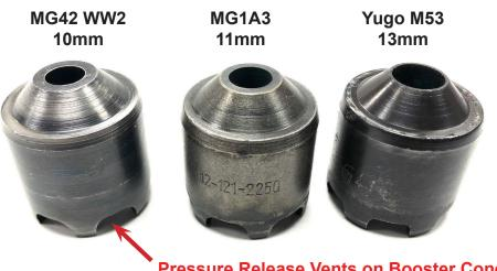
**Pressure Release Vents on Booster Cone**
