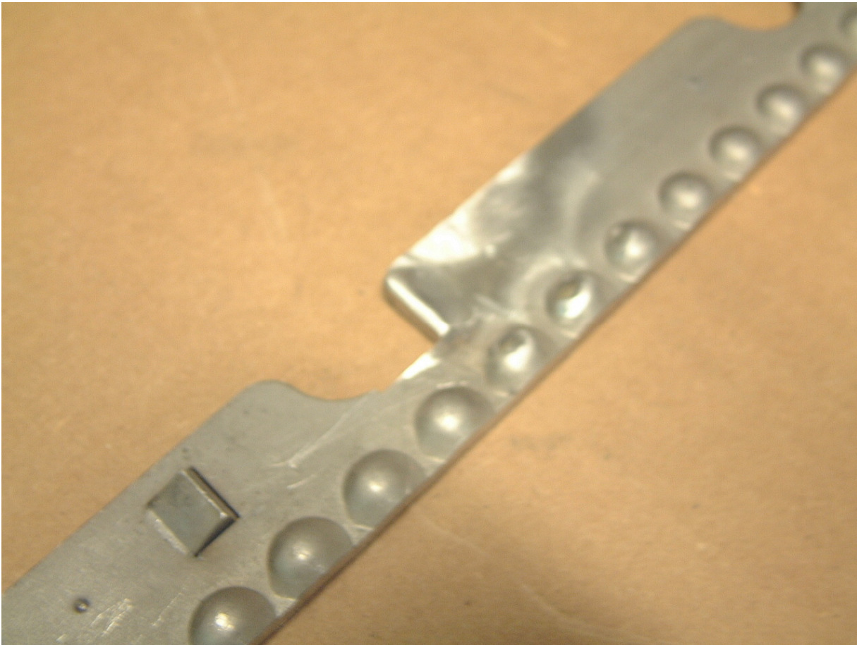
97- Grind the weld into a smooth ramp.
