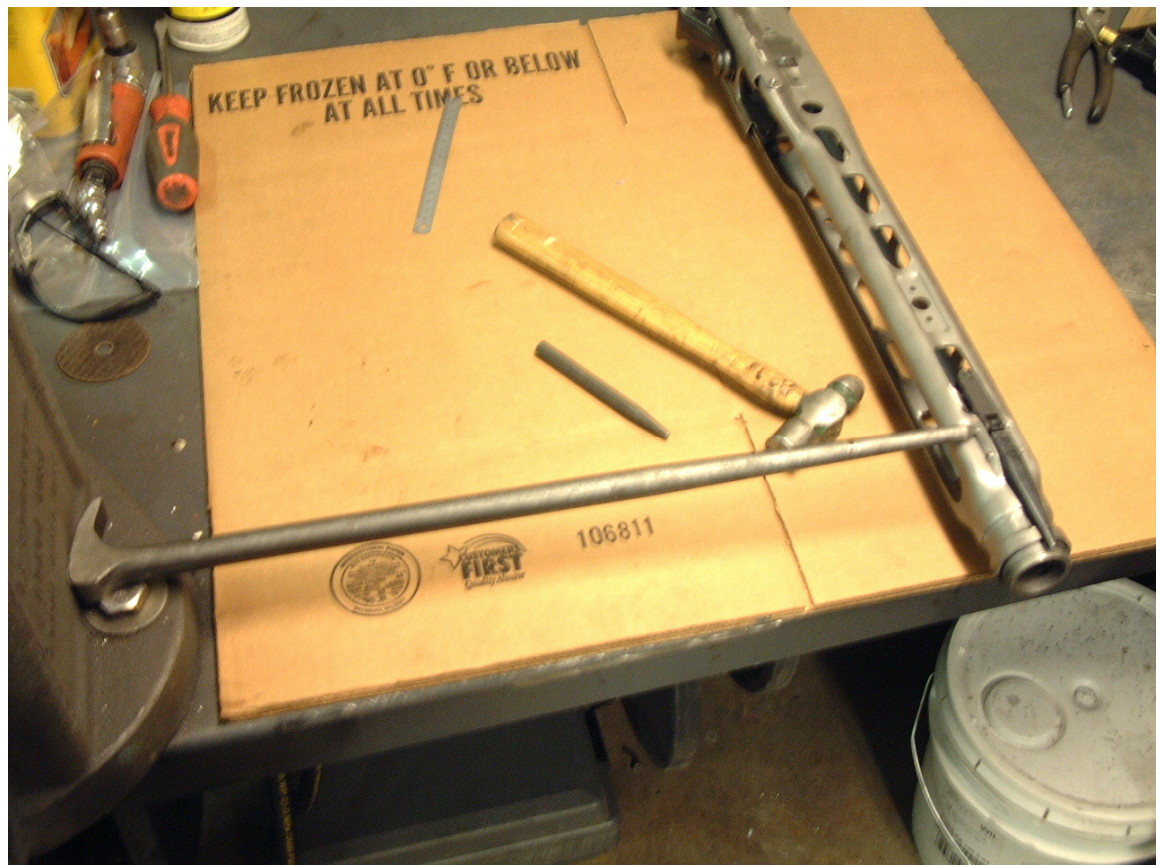
86- Mushroom both ends of the pins. A lady finger up against a vice on one side while hitting the other side works well.
