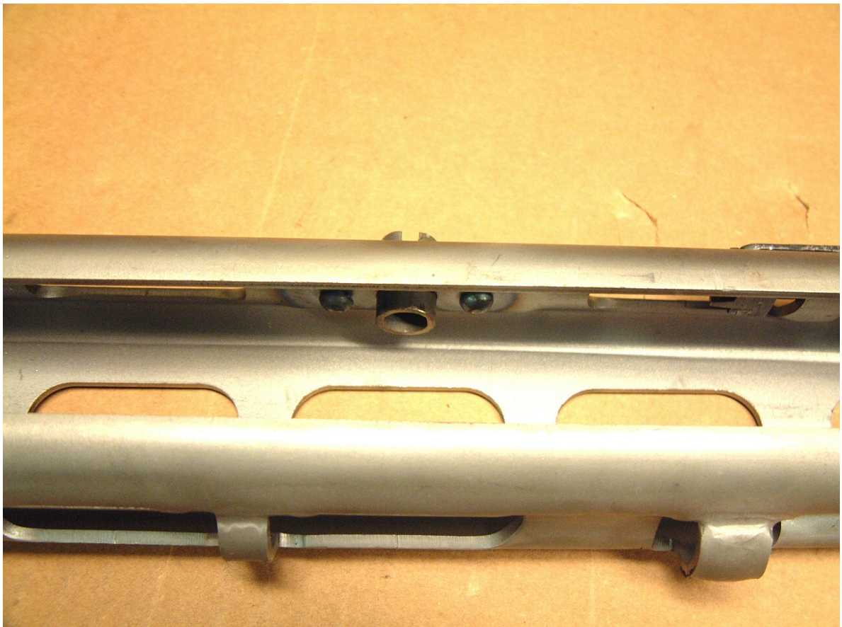
87- Install the front AA sight bracket. Insert the rivets from the inside. Rivet in place.
