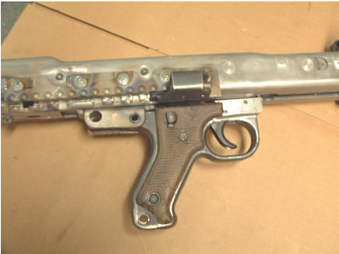
112- Ensure the charging handle is all the way forward in the receiver. Install the trigger pack. The hammer on the trigger pack must be down in the cocked position to install.
