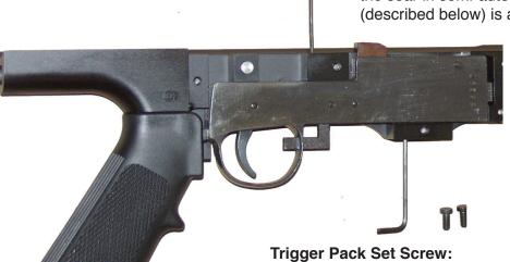
This is loosened to remove the trigger pack and tightened to keep the trigger pack firmly in the upmost position when assembled.
