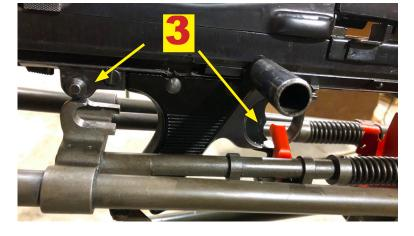
5) With the rear tripod pin fully seated in the claw, pull back the front tripod latch and allow the front mount bracket on the adapter to drop and lock into the front tripod mount.
