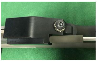
3) Align the trigger puller assembly on the trigger guard and attach to the lower housing using a 5/32 Allen wrench and the button head screw supplied. A lock washer is supplied to keep the mounting screw from backing off during use.
