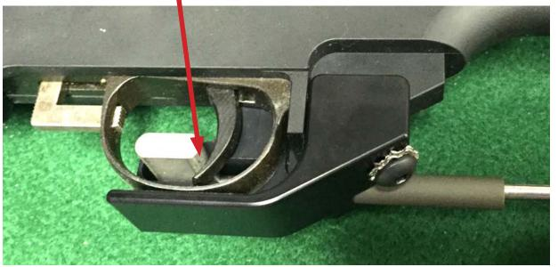
6) Slide the lock washer over the first 8-32 nut. With an 11/32" thin wrench or adjustable wrench, gently screw on the second 8-32 nut onto the back of the trigger connecting rod. Tighten carefully so you don't further move the first 8-32 nut and disturb the timing from the previous step.
