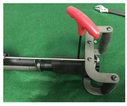
6) With an 11/32" thin wrench or adjustable wrench, gently screw on one of the 8-32 nut onto the back of the trigger connecting rod.
